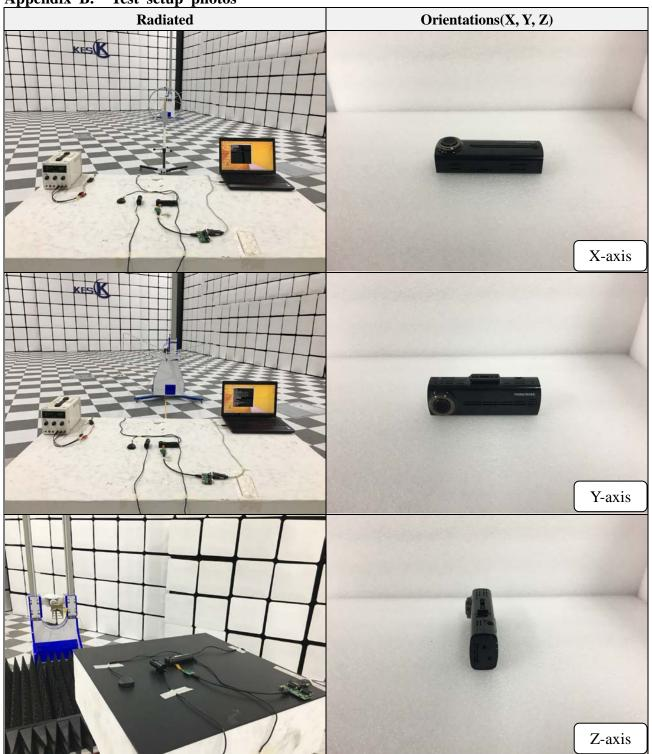
Note: Radiated testing was performed with the EUT in worst case X-axis.
