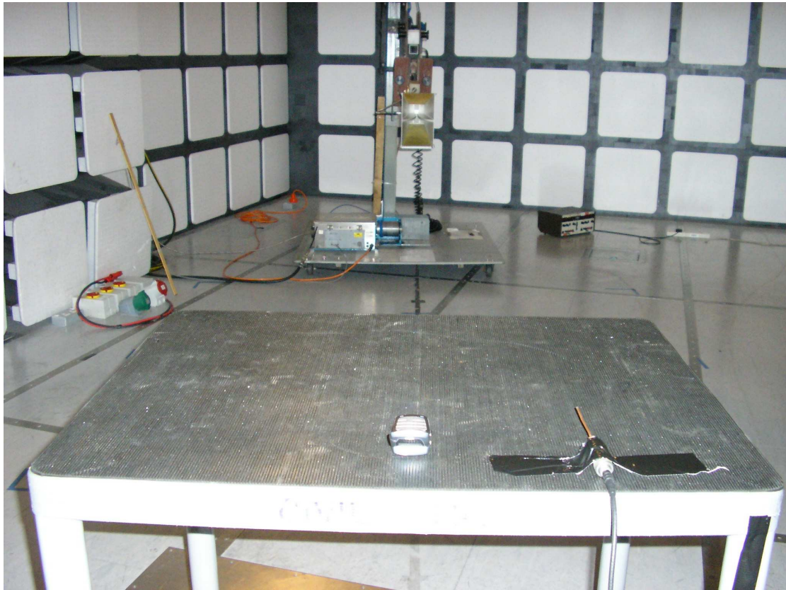
Sagem DC2006a – Test Set Up Photo 3 (Bluetooth Radiated Emissions)
