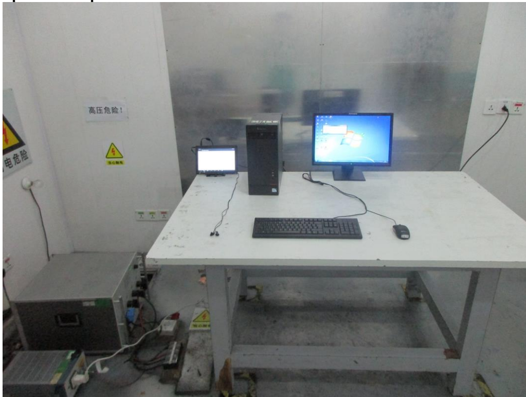
Photograph 2: Set-up for Radiated Emission of below 1GHz
