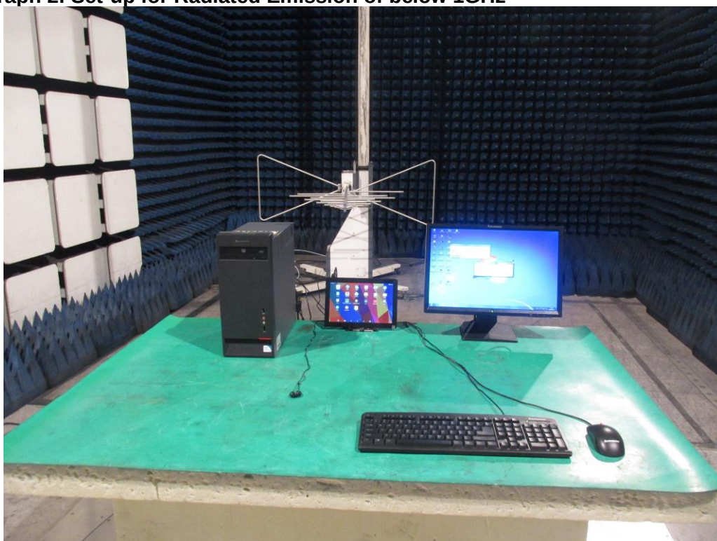
Photograph 2: Set-up for Radiated Emission of below 1GHz
