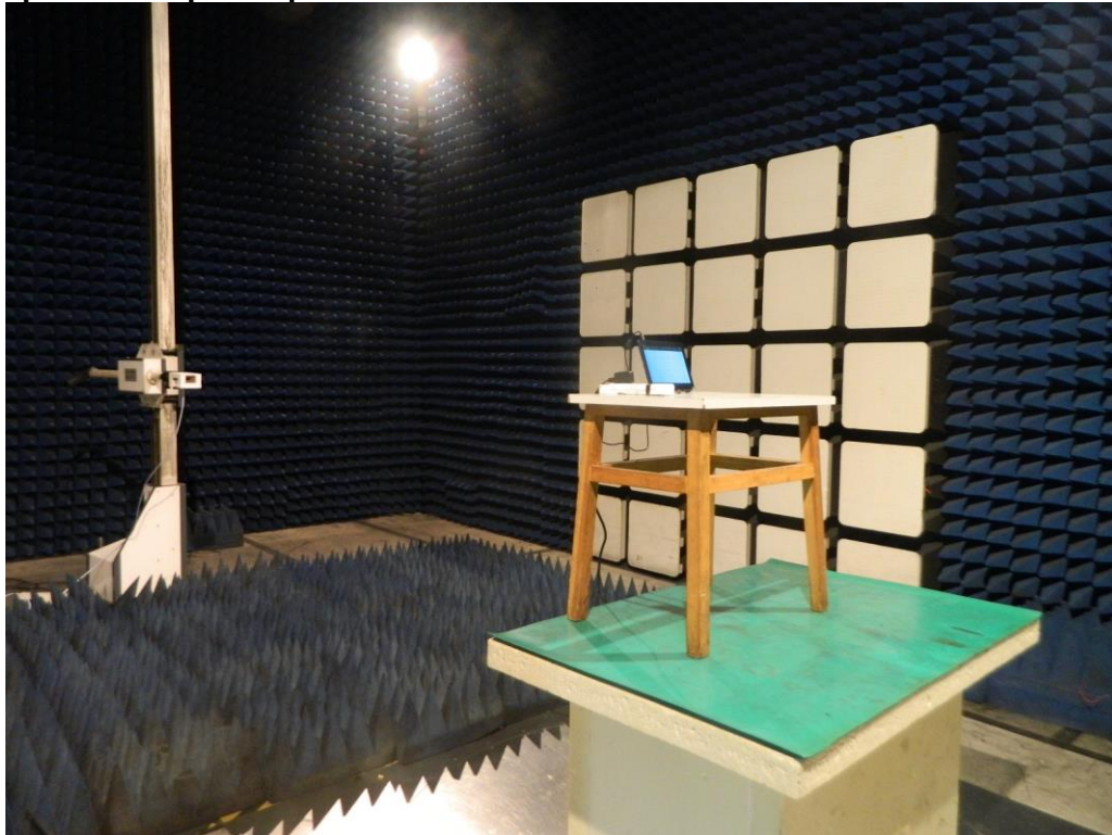
Photograph 5: Set-up for Spurious Emissions for 18 - 40GHz
