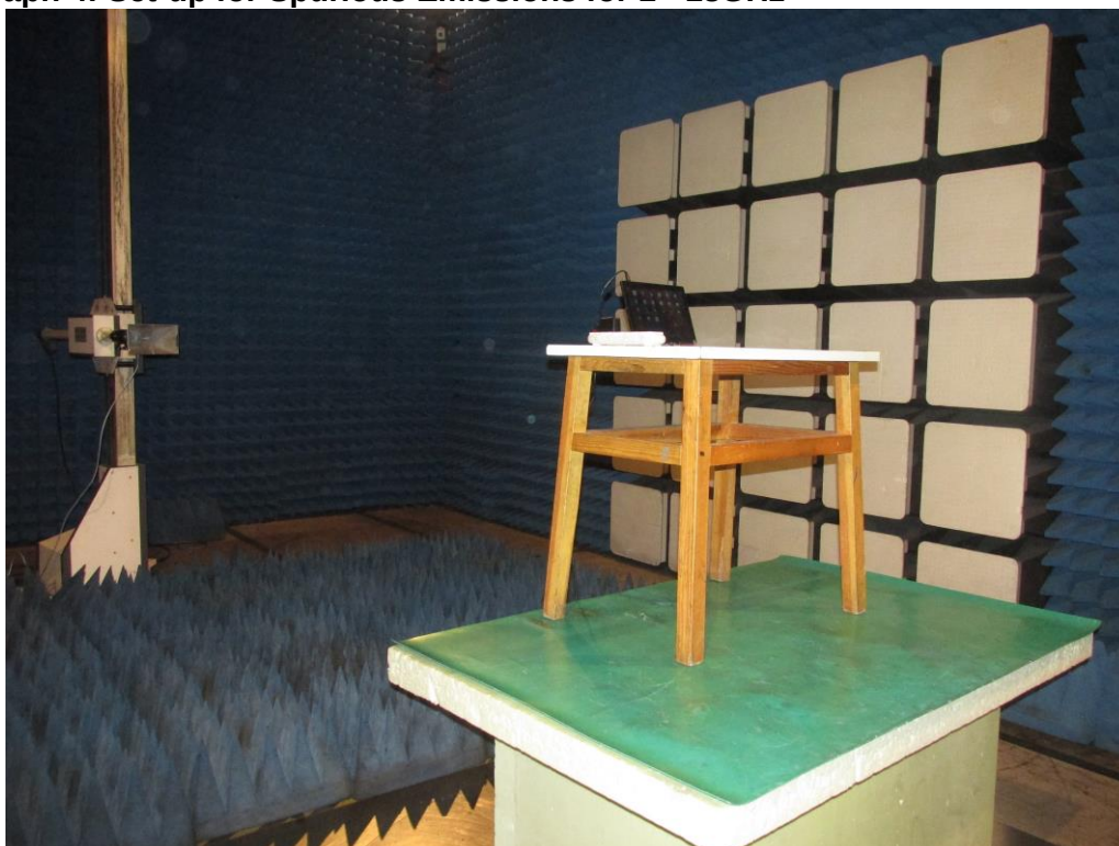
Photograph 4: Set-up for Spurious Emissions for 1 - 18GHz
