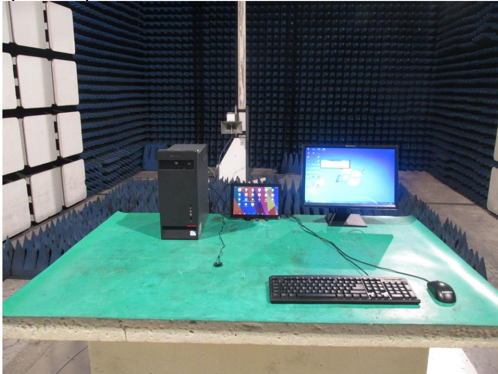
Photograph 3: Set-up for Radiated Emission of 1 - 18GHz
