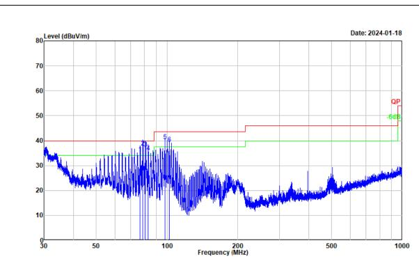
Project No. : RWAZ202300121-RF Test Mode : Transmitting Test Voltage : AC 120V/60Hz
