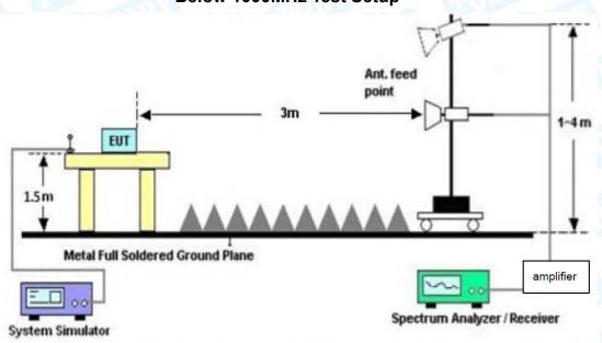
**Above 1GHz Test Setup**
