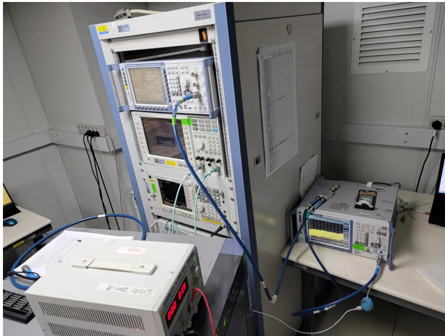
RF Conducted Test setup (GSM/WCDMA/LTE)
