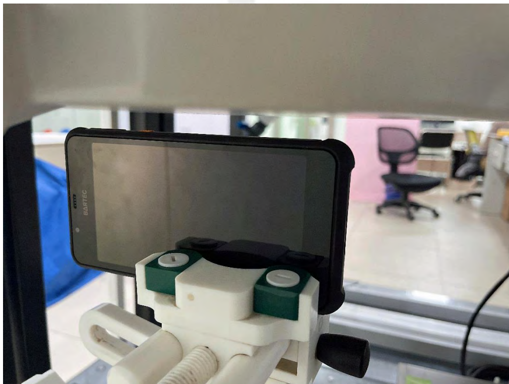
Body Right side(separation distance is 10mm)
