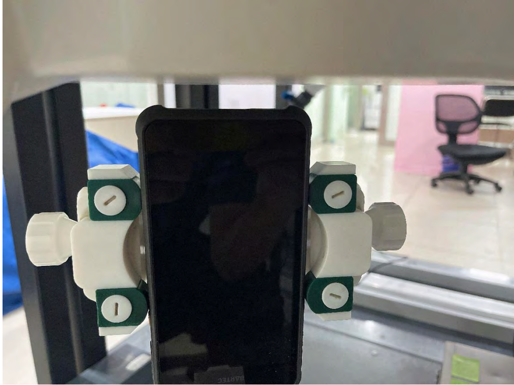
Body Bottom side(separation distance is 10mm)
