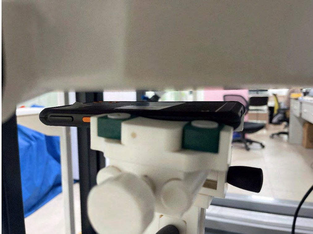
Body Front side(separation distance is 10mm)
