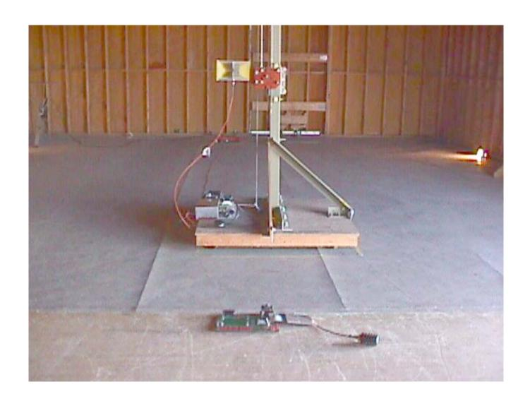
**EXHIBIT 9 - Test Setup Photos (Radiated Emissions Test Setup)**
