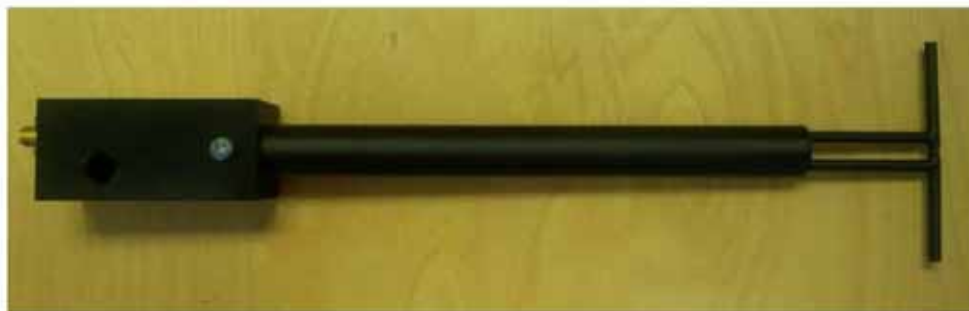
Figure 1 – MVG COMOSAR Validation Dipole
