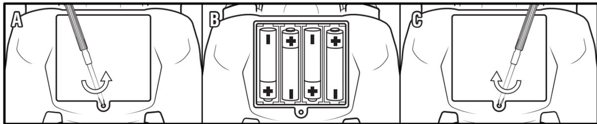
1. Open the battery door with a screwdriver (A). 2. If used batteries are present, remove these batteries from the unit by pulling up on one end of each battery. DO NOT remove or install batteries using sharp or metal tools. 3. Install new batteries as shown in the polarity diagram (+/-) inside the battery compartment (B). 4. Replace battery door securely (C). 5. Check your local laws and regulations for correct recycling and/or battery disposal.
