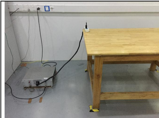
Conducted Emissions Test Setup – Front View
