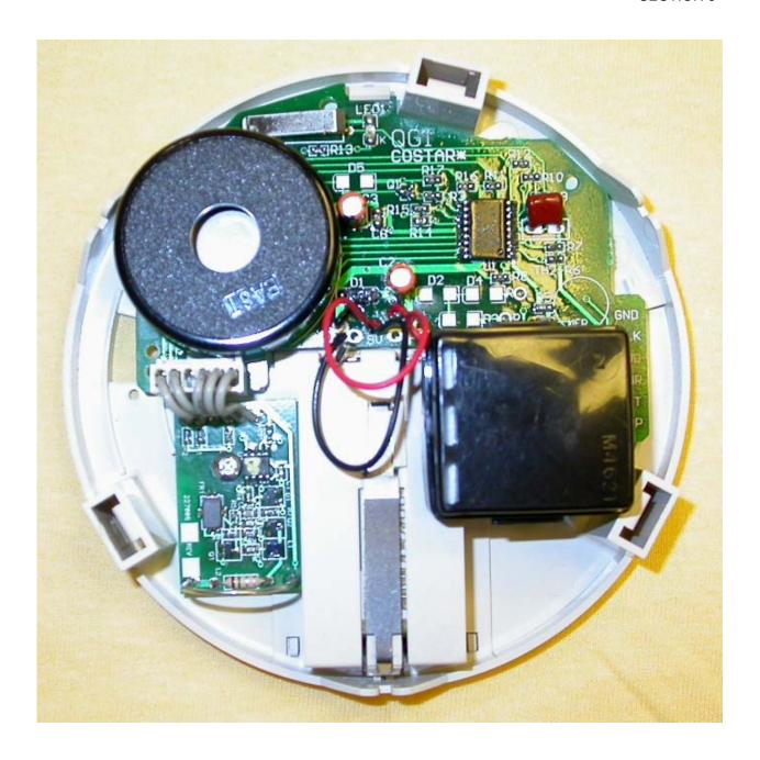
INTERNAL PCB LAYOUT WITH RF TRANSMITTER PCB
