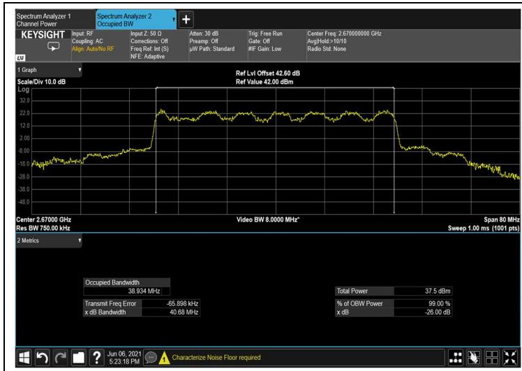
**Figure 143: output 16QAM 40MHz B.W.; 2670.0MHz, 15kHz**
