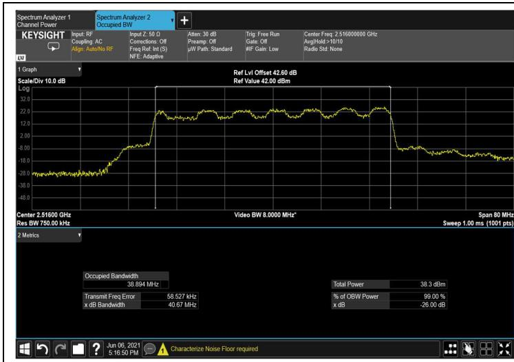
**Figure 137: output 16QAM 40MHz B.W.; 2516.0MHz, 15kHz**
