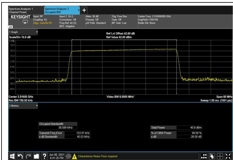
**Figure 152: output 64QAM 40MHz B.W.; 2516.0MHz, 15kHz**
