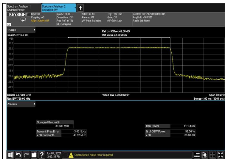
Figure 113: input 256QAM 40MHz B.W.; 2670.0MHz, 15kHz
