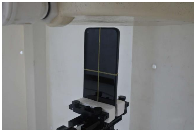
Top Side, Test Separation 10 mm
