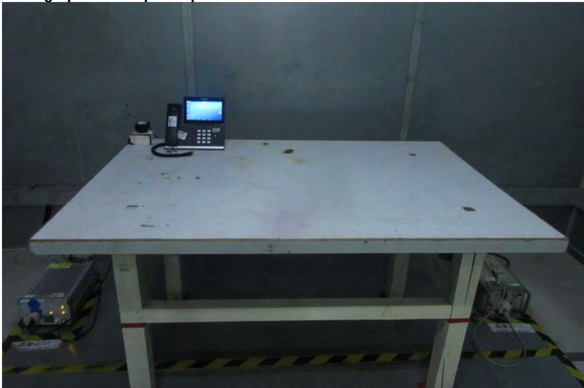
Photograph 4: Set-up for Spurious Conducted Emissions
