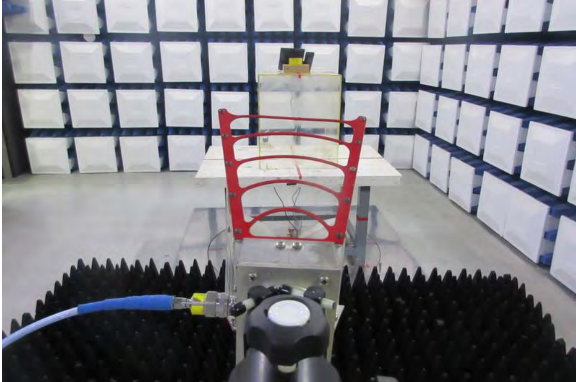
Photograph 4: Set-up for Spurious Conducted Emissions
