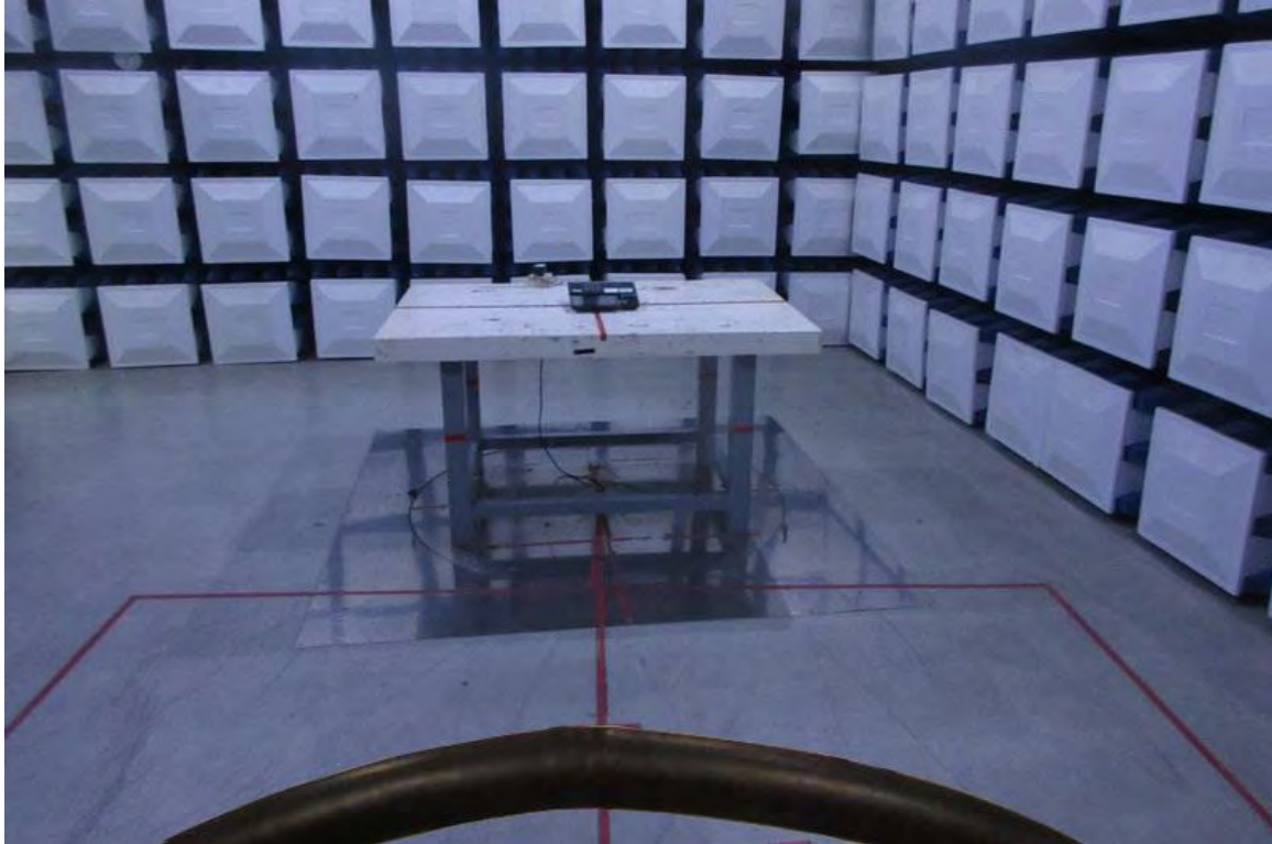
Photograph 2: Set-up for Spurious Emissions for 30 - 1000MHz
