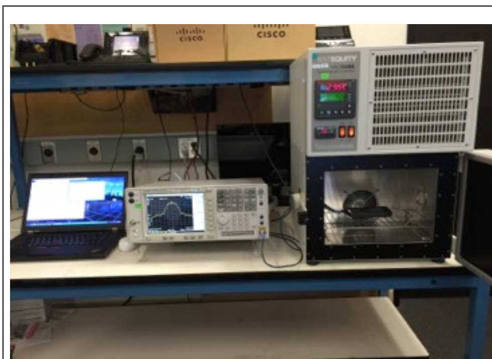
Title: Temperature / Frequency Stability Test Set Up
