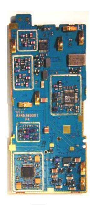
RF board without Shields (Bottom)
