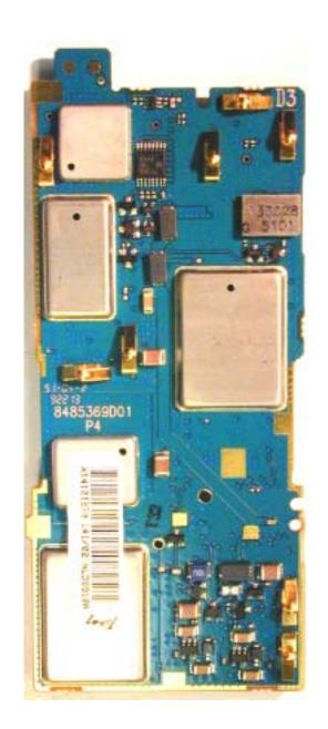
RF board with Shields (Bottom)
