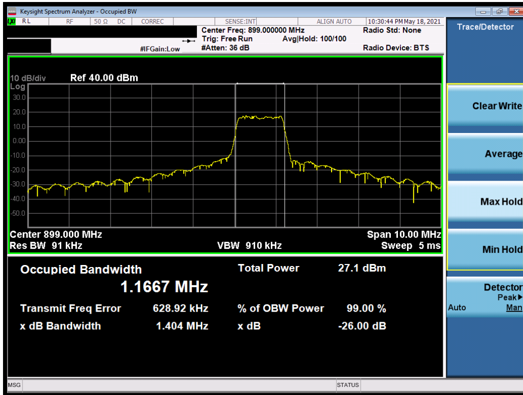
Plot 7-2. Occupied Bandwidth Plot (3MHz, QPSK, RB 6, RB Offset 0, NB=1)
