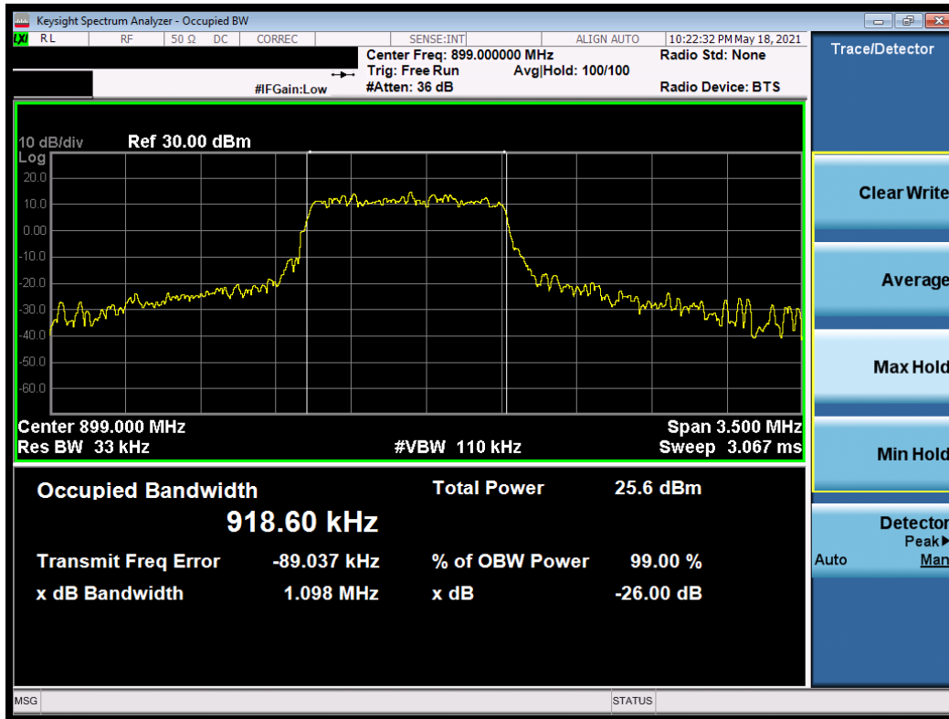
Plot 7-8. Occupied Bandwidth Plot (1.4MHz, 16-QAM, RB 5, RB Offset 0, NB=0)
