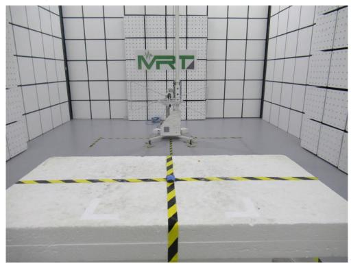
Description: Radiated Spurious Emission Test Setup for Between 1  $\sim$  18GHz
