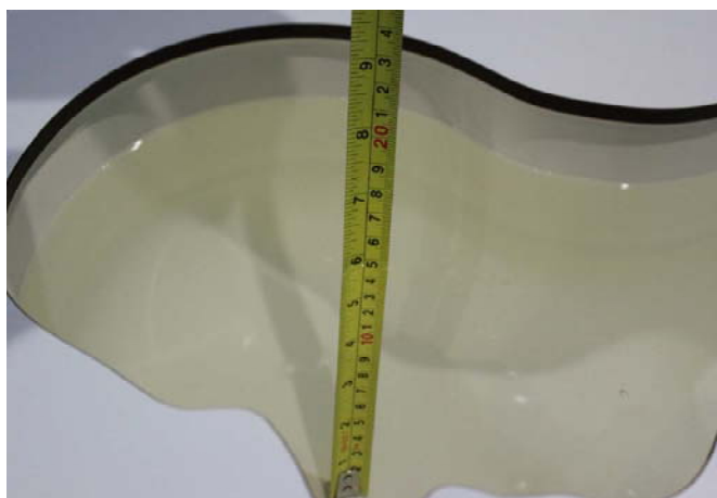
Liquid depth in the head phantom (5GHz)
