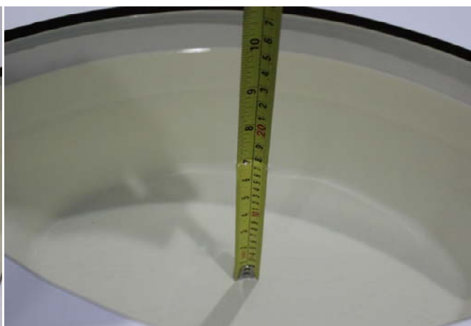
Liquid depth in the body phantom (5GHz)
