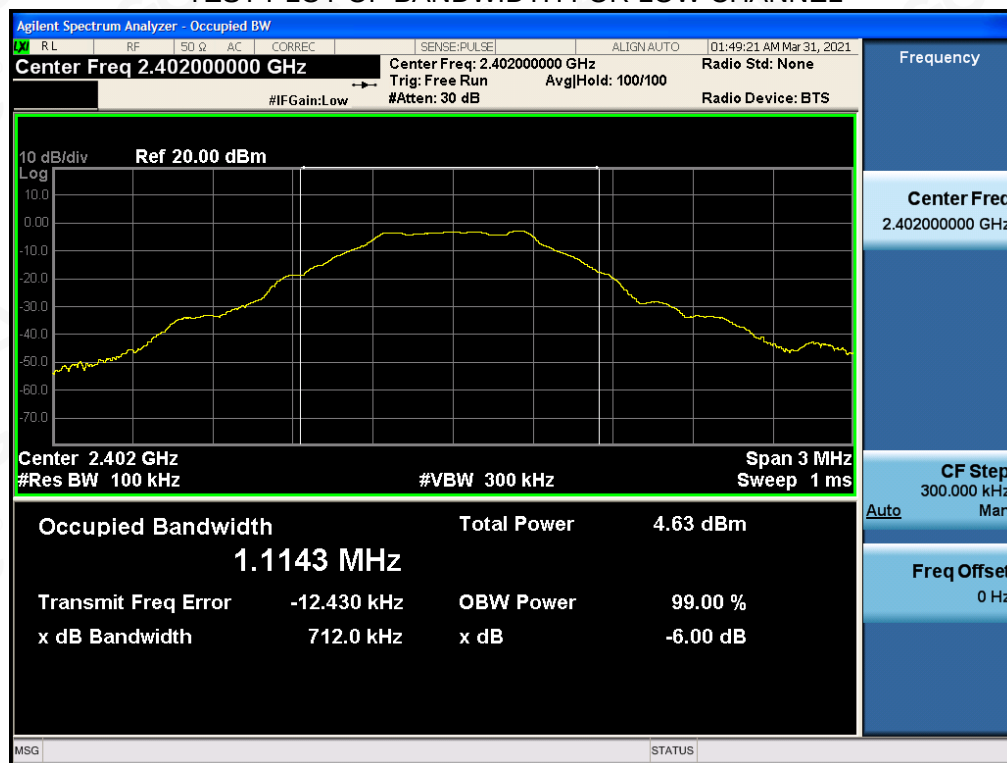
TEST PLOT OF BANDWIDTH FOR LOW CHANNEL
