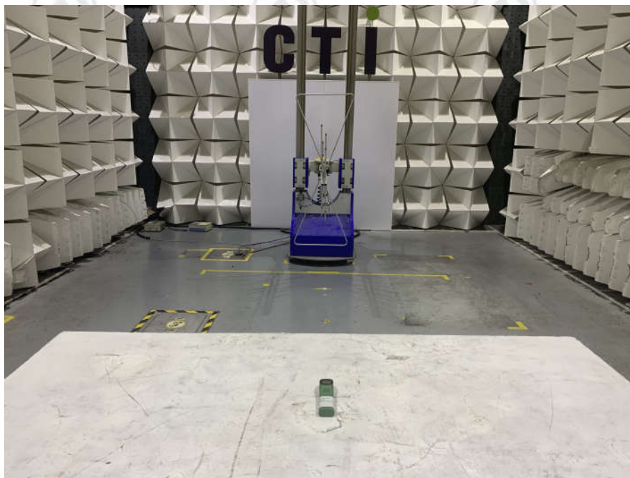
Radiated spurious emission Test Setup-1(Below 1GHz)
