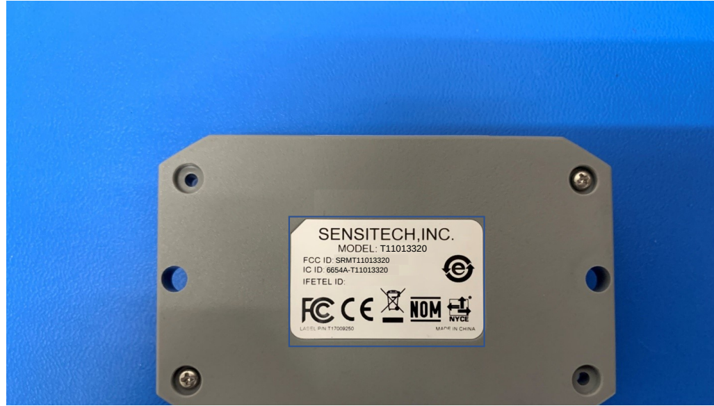
Sensor FCC label location
