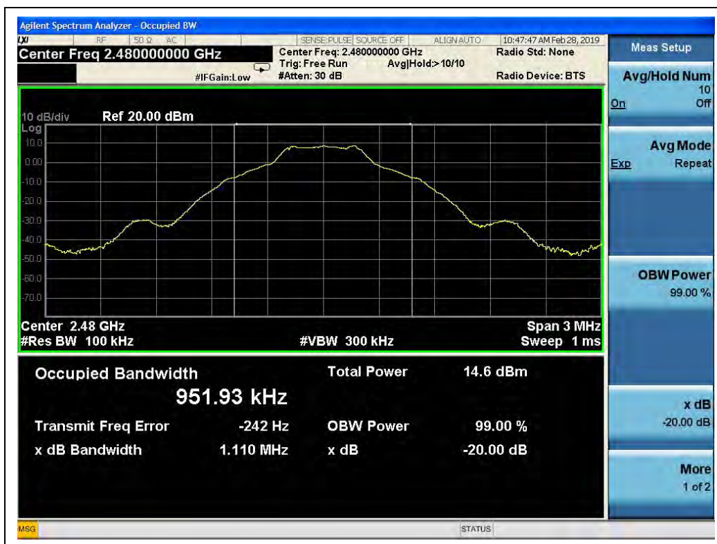
(GFSK, Channel 78, 2480MHz)
