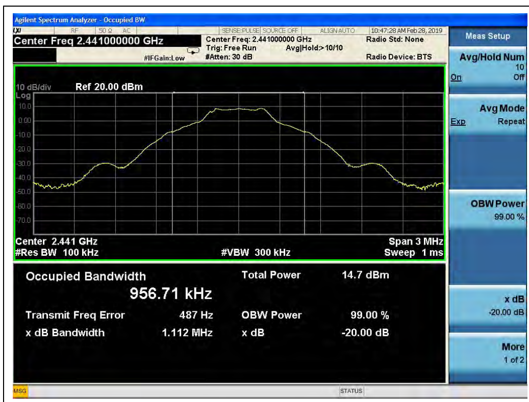
(GFSK, Channel 39, 2441MHz)
