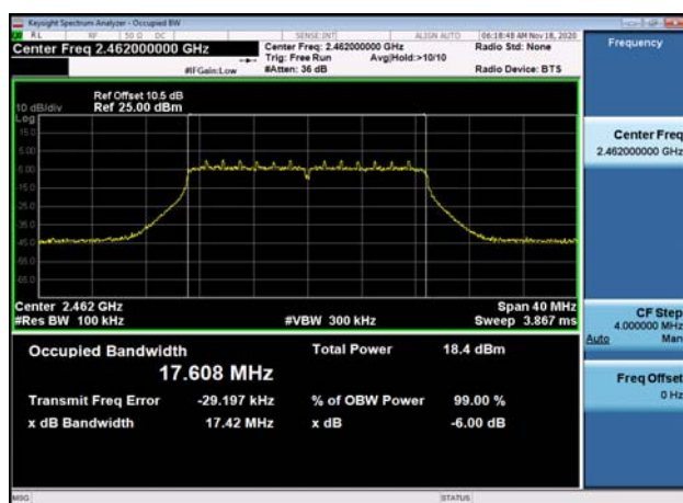
6dB Bandwidth-802.11n(HT40),2437MHz
