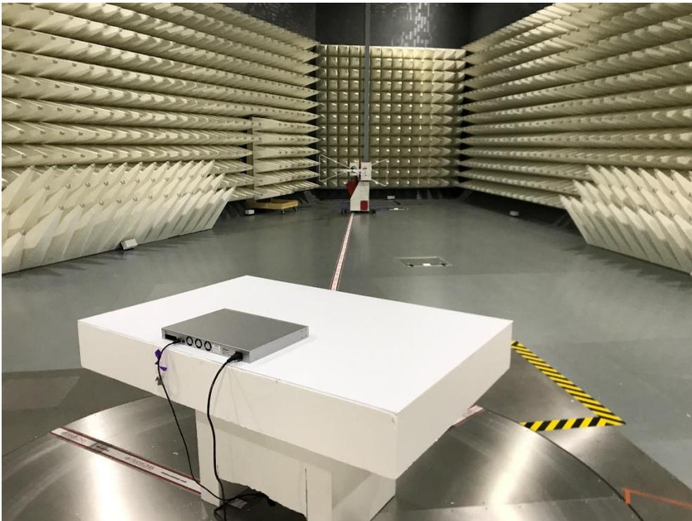
**Photograph 2: Back View Test Set Up 30 – 1000 MHz**
