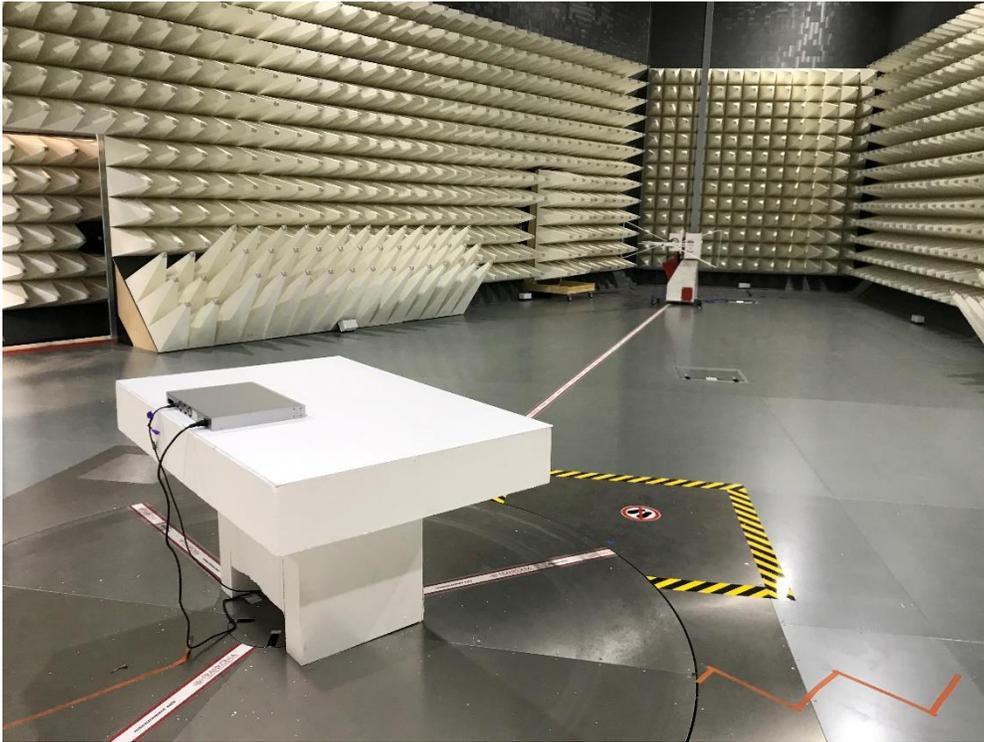
**Photograph 1: Side View Test Set Up 30 – 1000 MHz**
