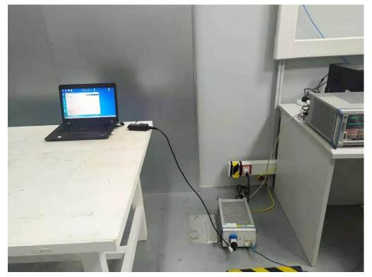
Radiated emission test 30MHz – 1GHz
