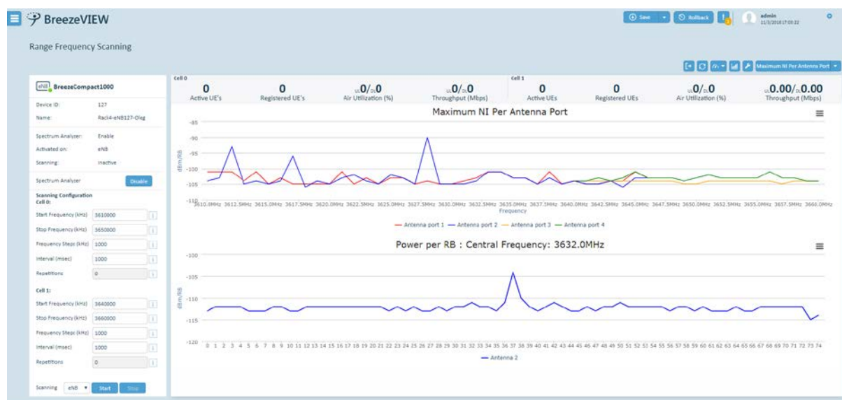
Figure 91: BREEZVIEW -ENB Spectrum Analyzer Range Frequency Scanning page
