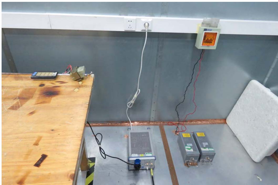
Picture 2 Conducted Emission Test Setup
