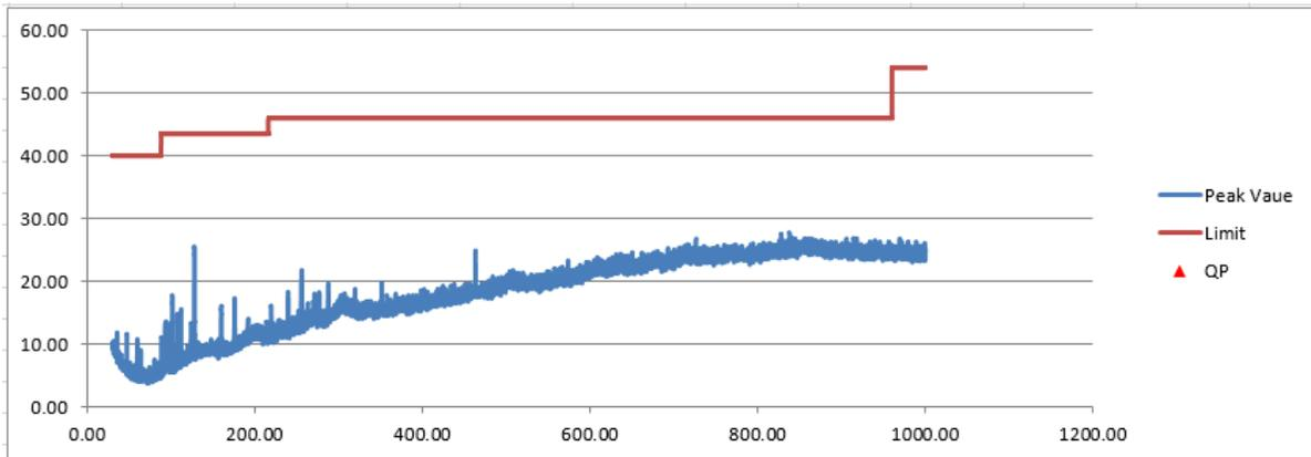
**Figure 3. Radiated Emissions Graphical Data, 30-1000 MHz – Horizontal**
