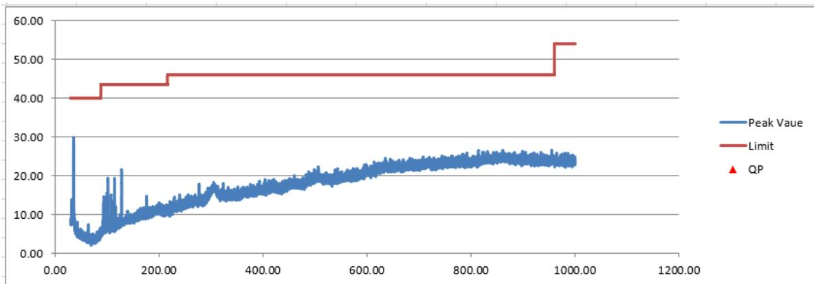
**Figure 4. Radiated Emissions Graphical Data, 30-1000 MHz – Vertical**
