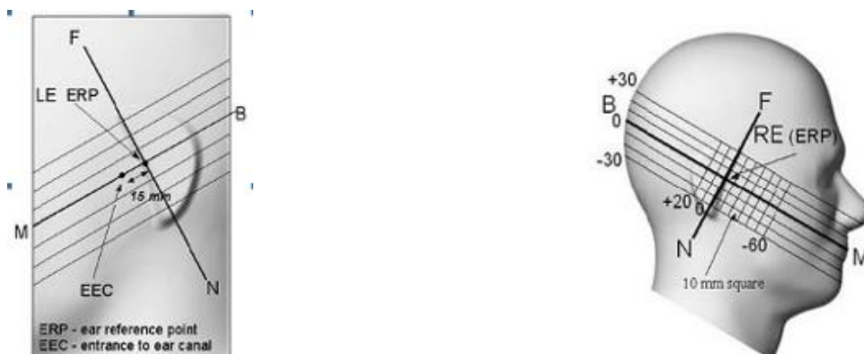
F-4. Sagittally bisected phantom with extended perimeter (shown placed on its side as used for SAR measurements)
