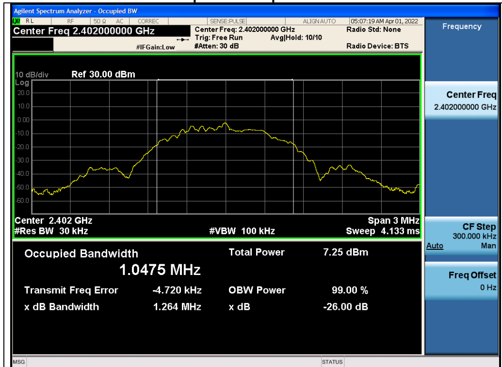
Test_Graph_LE1M_ANT2_2402_1Mbps_OBW
