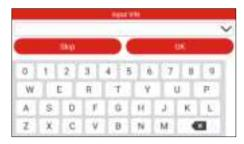
Input the VIN, and tap "OK", the system will decode the VIN data automatically, and continue the Smart Diagnosis procedure if success. Otherwise the system will enter the Manual Diagnosis mode.
