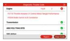
In above figure, the tested system with fault code is tagged with a red cross and the system with OK displays with a green tick.
