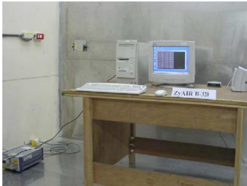
Photo 2: Conducted Emission Test Set-up
