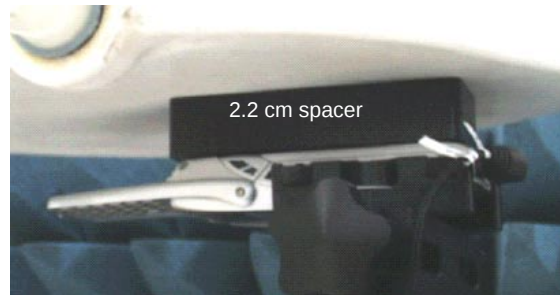
Photos of the device positioned for Body SAR measurement with flip closed and with flip open. The spacer was removed for the tests.
