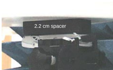
Photos of the device positioned for Body SAR measurement with flip closed and with flip open. The spacer was removed for the tests.
