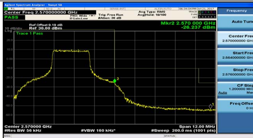
(Channel Bandwidth: 5 MHz)_HCH_QPSK_12RB#13
