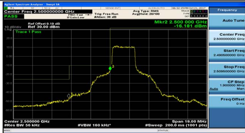
(Channel Bandwidth: 5 MHz)_LCH_QPSK_12RB#6
