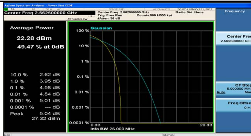
(Channel Bandwidth:15 MHz)_HCH_16QAM_75RB#0
