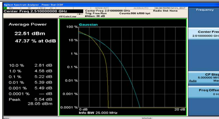
(Channel Bandwidth:20 MHz)_LCH_16QAM_100RB#0
