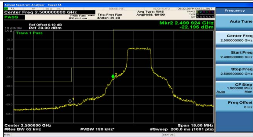
(Channel Bandwidth: 5 MHz)_LCH_QPSK_12RB#13
