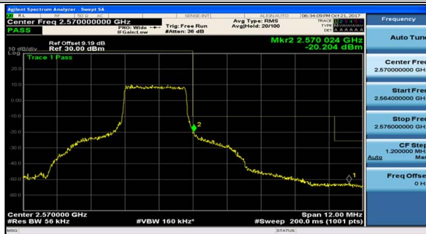
(Channel Bandwidth: 5 MHz)_HCH_QPSK_25RB#0
