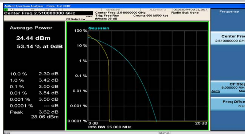
(Channel Bandwidth:20 MHz)_LCH_QPSK_50RB#0
