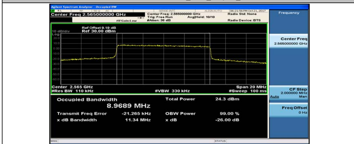
Channel Bandwidth: 10 MHz_HCH_16QAM_50RB#0
