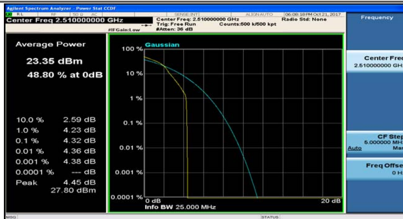
(Channel Bandwidth:20 MHz)_LCH_16QAM_50RB#0
