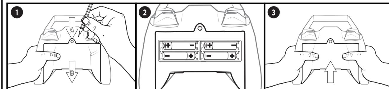
**EN** 1. Press down on release button (A) to slide down battery cover (B). 2. If used batteries are present, remove these batteries from the unit by pulling up on one end of each battery. DO NOT remove or install batteries using sharp or metal tools. Install new batteries as shown in the polarity diagram (+/-) inside the battery compartment. 3. Replace battery door securely. **NOTE:** Check your local laws and regulations for correct recycling and/or battery disposal.
