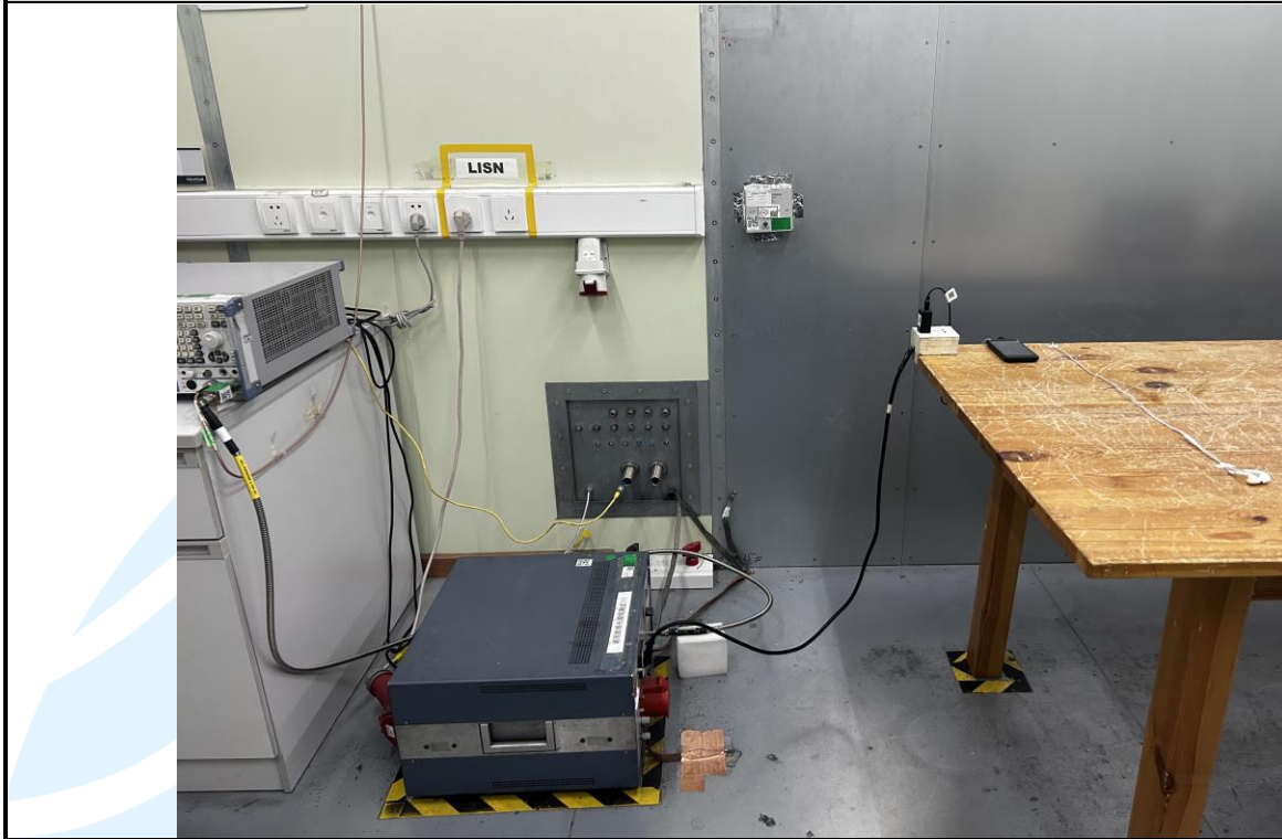
Conducted Emission Test Setup
