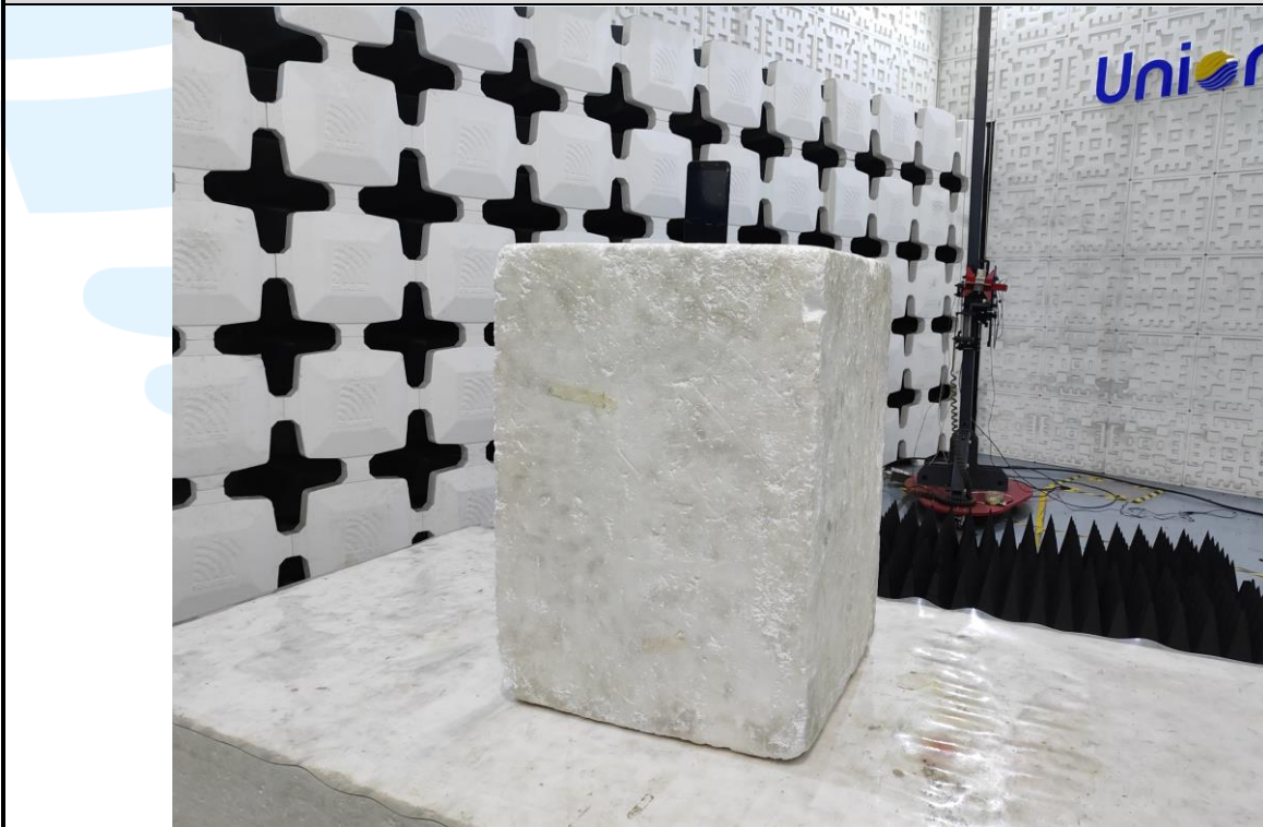
Radiated emission Test Setup (Above 1 GHz)
