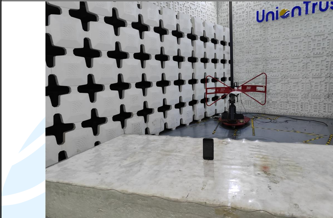
Radiated emission Test Setup (30 MHz~1 GHz)
