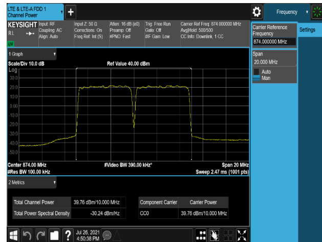
Plot 7-141. Conducted Average Output Power Plot (LTE_B5_5M+5M_2C_QPSK - Low Channel, Port 3)
