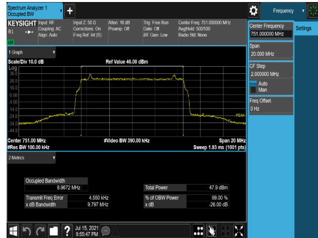
Plot 7-76. Occupied Bandwidth Plot (LTE_B13_10M+Low_NB-lot(IB)+High_NB-lot(IB)_1C_QPSK - Port 1)
