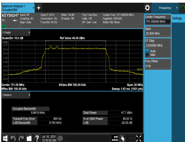
Plot 7-77. Occupied Bandwidth Plot (LTE_B13_10M+Low_NB-lot(IB)+Low_NB-lot(IB)_1C_QPSK-Port 0)
