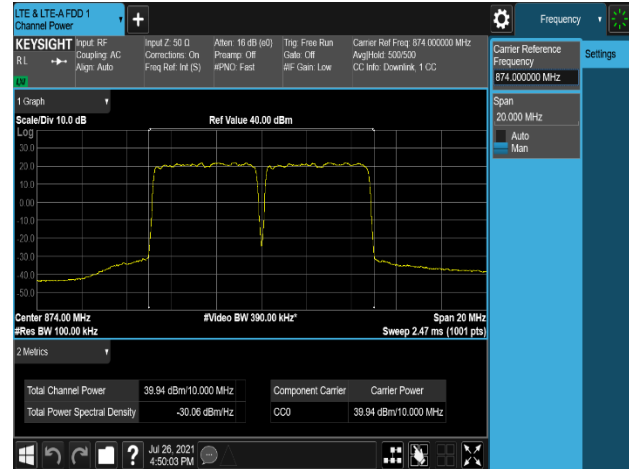
Plot 7-139. Conducted Average Output Power Plot (LTE_B5_5M+5M_2C_QPSK - Low Channel, Port 1)
