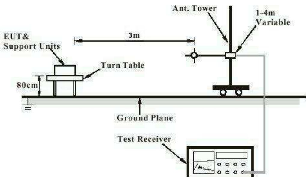
Note: Measurements above 1 GHz are done with a table height of 1.5m
