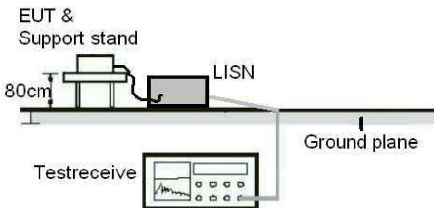
**Diagram of Measurement Equipment Configuration for Conducted Transmitter Measurement**
