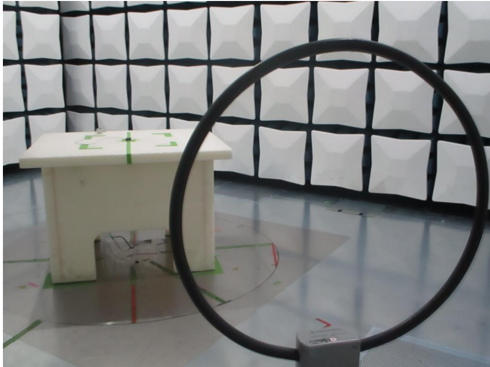
Figure 23: 9kHz-30MHz Test Setup (Front View)
