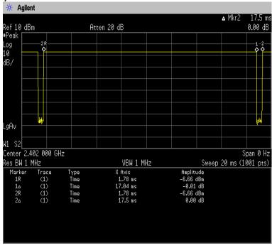
Duty Cycle = Ton / (Ton + Toff) =  $17040[\mu s] / (17040[\mu s] + 460[\mu s]) = 97.37[\%]$
