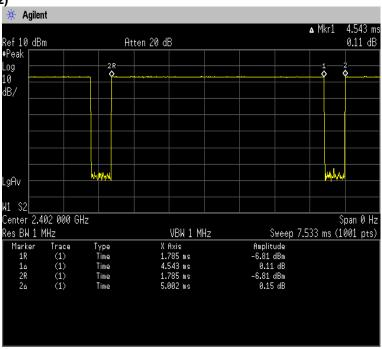
Duty Cycle = Ton / (Ton + Toff) =  $4543[\mu s]$  / ( $4543[\mu s]$  +  $459[\mu s]$ ) = 90.82[%]
