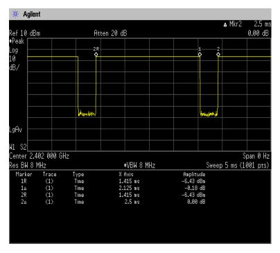
Duty Cycle = Ton / (Ton + Toff) =  $2125[\mu s] / (2125[\mu s] + 375[\mu s]) = 85[\%]$
