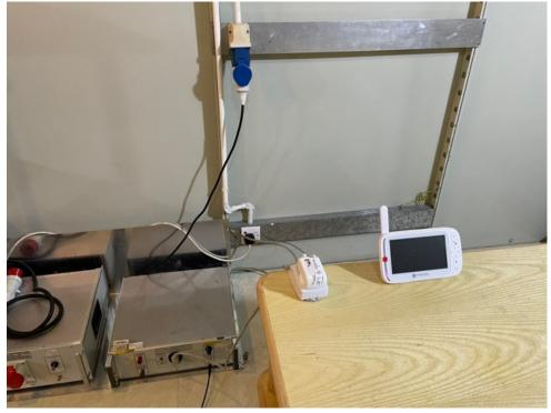
Radiated Emissions (30MHz-1GHz) Test Setup
