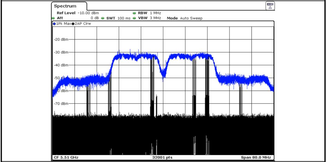
**EUT (Client ) links with master on 5510MHz**
