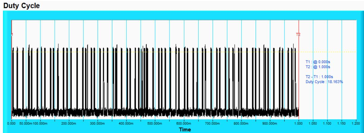
**NOTE:** T1 denotes the start of duty cycle period is 0th second. T2 denotes the end of duty cycle period is 1th second. T2 – T1= 1 seconds. Duty Cycle = 18.163%.
