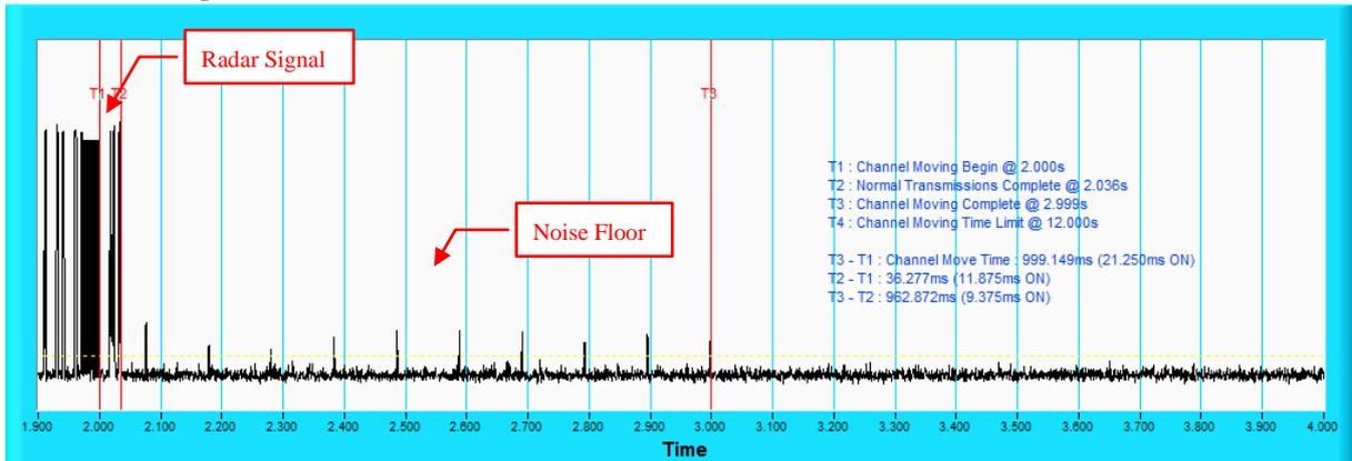
**NOTE:** Zoom in of the first 2000ms after radar signal applied.
