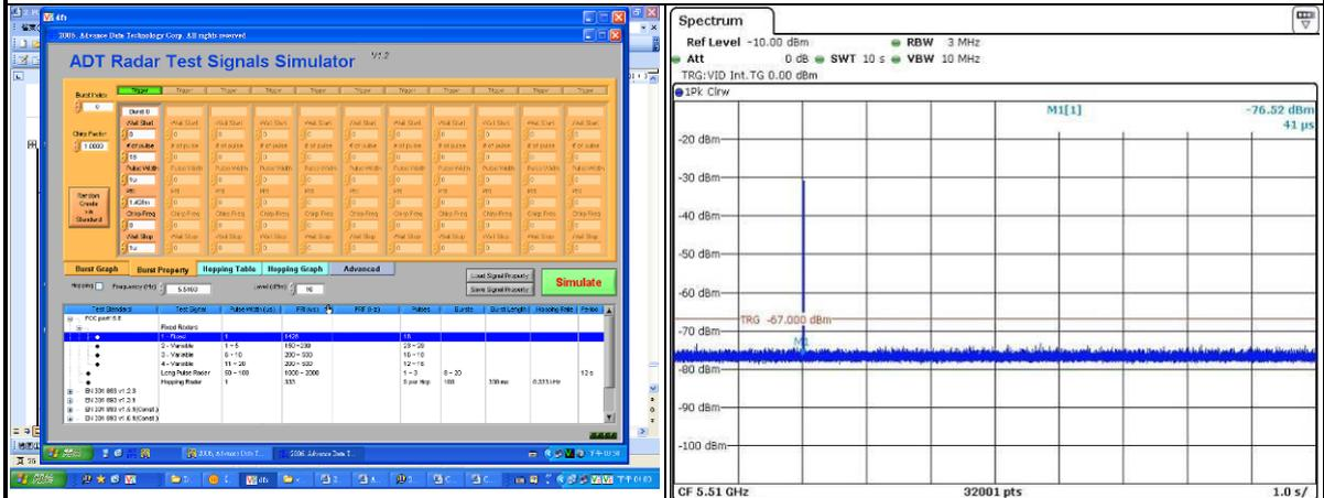
Radar Signal (Type 0) is used to test during DFS testing.
