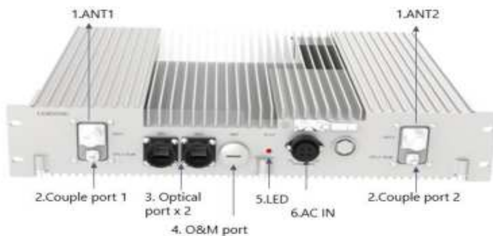
Figure 24. dMRU Interfaces
