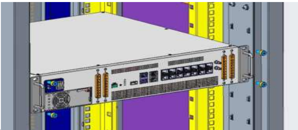
Figure 36. Installation Diagram of DCU in the Rack
