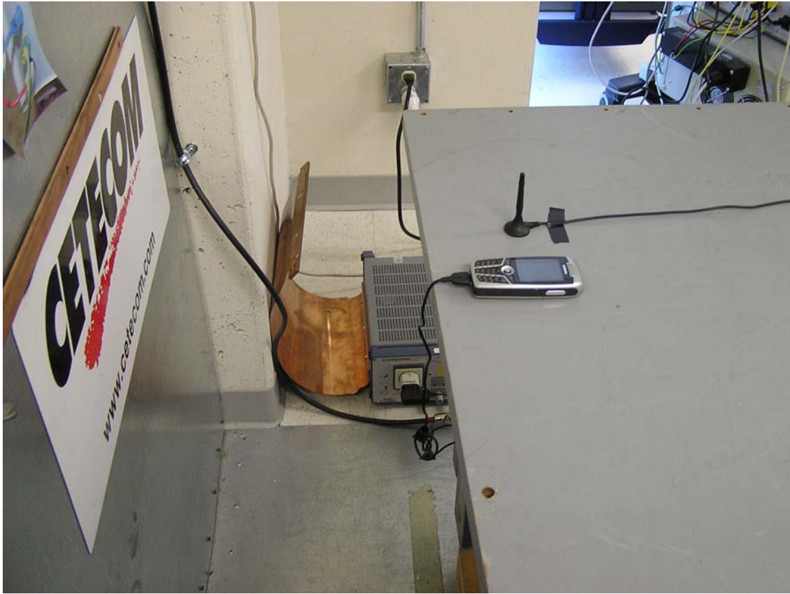
Test setup – AC Line conducted measurements
