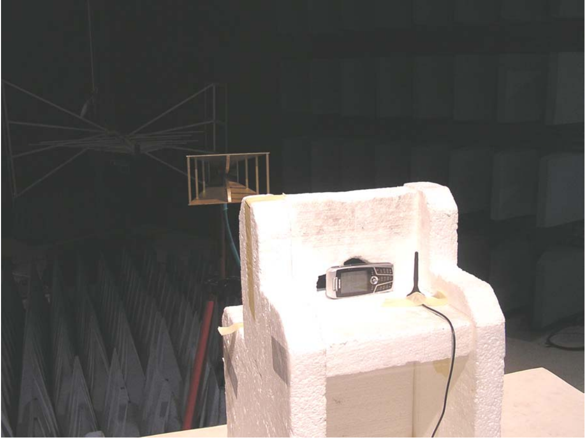
Test setup – Radiated Emissions
