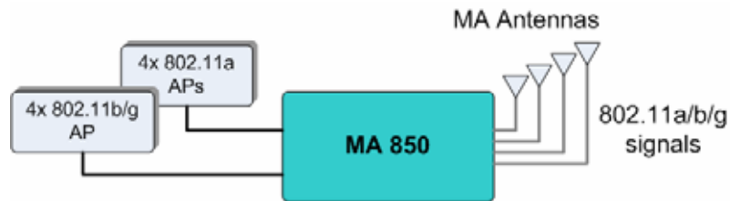
Figure 1-3. MA 850 Standalone Installation Configuration
