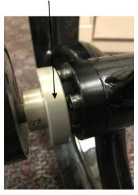
Wheel is installed on the second groove. The cart will now move using the motors. Notice the wheel sits flush against the axle hub:
