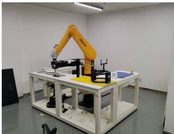
Picture D.6 Specific Absorption Rate Test Layout
