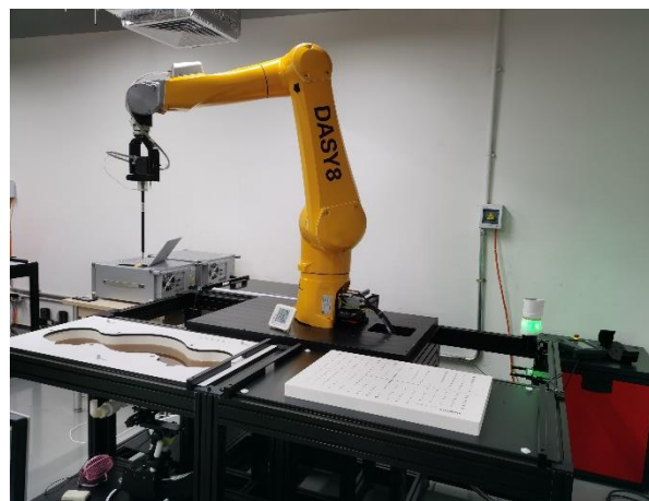
Picture D.6 Specific Absorption Rate Test Layout
