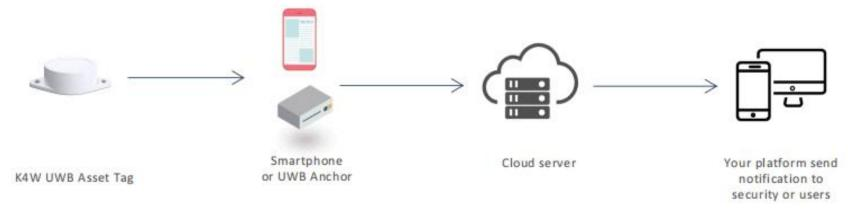
Using the app/UWB Anchor to scan/connect the K4W' signal, then the APP/Anchor receivd its data and handle the data to reach the location usage.
